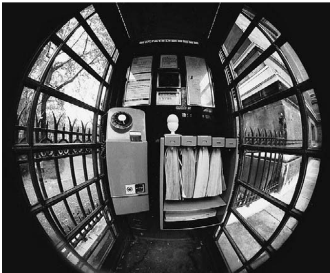
Figure 5.13 Fish-eye lens distortion. Inside an antique British telephone box, taken with a 35 mm camera and an 8 mm fish-eye lens designed to give a 220° angle of view. This extreme lens forms a circular picture with vertical and horizontal lines increasingly bowed according to their distance from the centre
