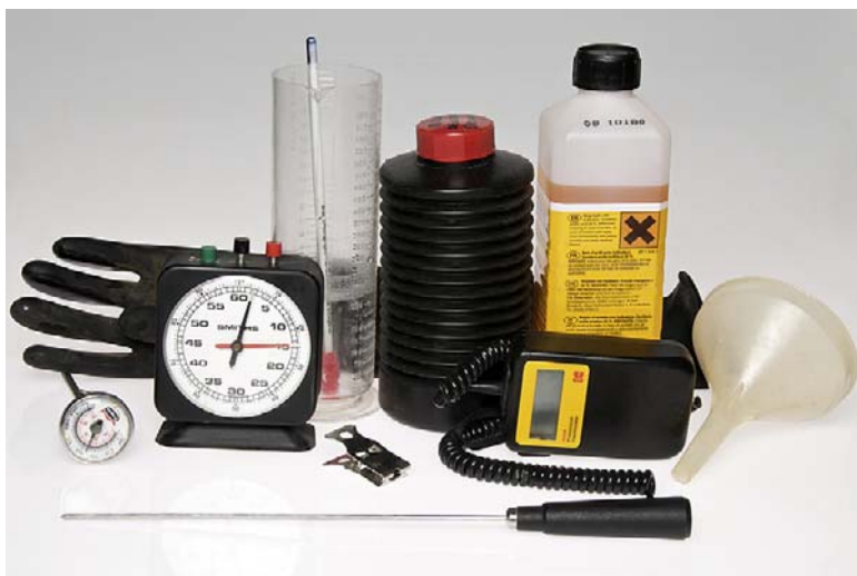
Figure 11.3 Left to right: Thermometer dial type, protective latex gloves, minutes/seconds timer, graduate and mixing rod for mixing and diluting, clip for hanging up film, solution storage containers, thermometer (electronic digital), funnel.
