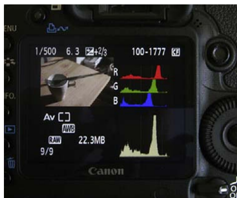
Figure 14.24 Almost every digital camera, whether compact or digital SLR, has the ability to display a histogram on-the-go, which is a handy way of quickly reviewing whether your photograph has been properly exposed. You can review it either as you are photographing or afterwards. Some models project the histogram onto the LCD giving you immediate feedback as you frame your picture
