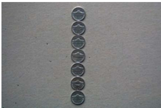
FIGURE 4.86 1:7 magnification ratio of a 50mm lens.
