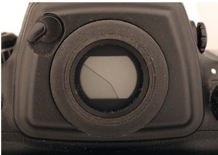
FIGURE 3.103B Newer Nikon cameras have built-in viewfinder covers. (Courtesy of Ron Taniwaki, Nikon Forensic Services.)
