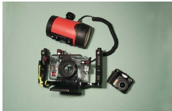
FIGURE 9.52 Underwater camera housing, flat port. (Courtesy of Nancy Olds, Forensic Photographer, United States Secret Service.)
