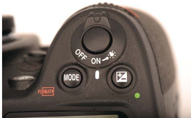
FIGURE 3.82B Exposure compensation button +/- on newer camera. (Courtesy of Ron Taniwaki, Nikon Forensic Services.)
