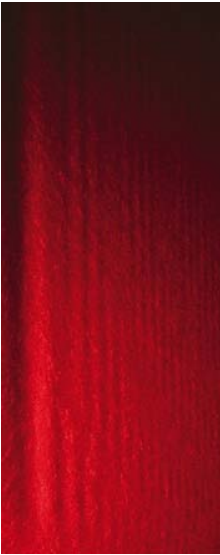
FIGURE 4.118 Diffraction pattern around a linear opaque edge.
