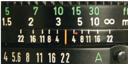
FIGURE 4.17 DOF scale: pairs of numbers opposite the orange line.
