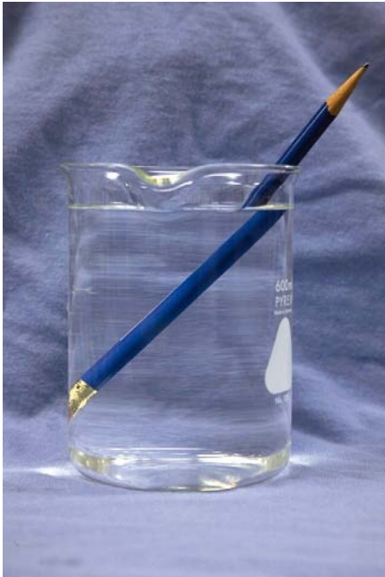
FIGURE 9.49 Refraction bending and magnifying a pencil.
