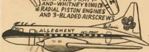
THE NAPIER ELAND TURBOLINER CONVAIR 540—LEASED TO ALLEGHENY AIRLINES OF THE EAST COAST IN 1959 AS A MODIFICATION OF THE 340, AND FOR THE FIRST TIME CONVERTED TO TURBINE POWER.
